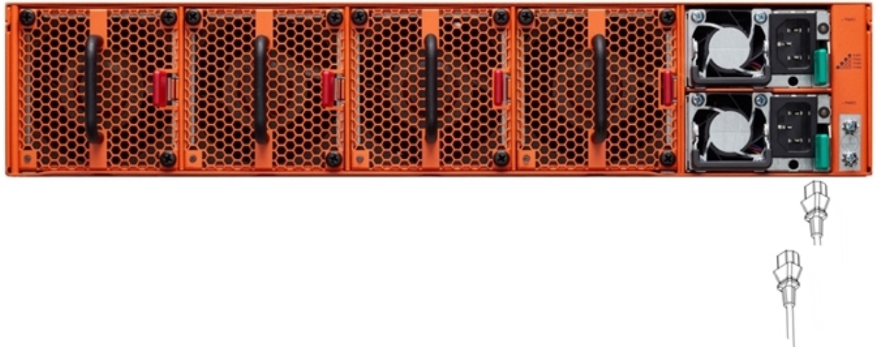
Figure 12 Connecting AC Power on a GigaVUE TA Series-TA200
